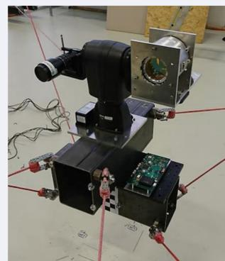
Figure 4 – cable robot sea state testing
