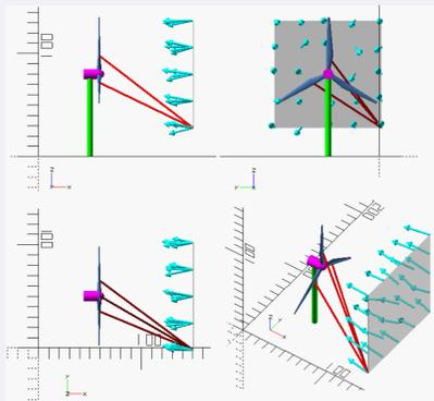
Figure 1 –forward looking 3d wind mapping/ scanning
